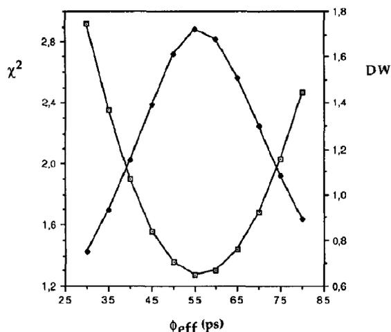
Fig. 5. Analysis of fluorescence anisotropy decay of lumiflavin according to a prolate ellipsoidal rotor. The experiment detailed in fig. 3A was analyzed using the parameters summarized in table 3. The effective correlation time,  $\phi_{\text{eff}}$ , was systematically varied until an optimum fit was obtained ( $\phi_{\text{eff}}=55$  ps). See text for details (●●●)  $\chi^2$  and (□□□) DW.
