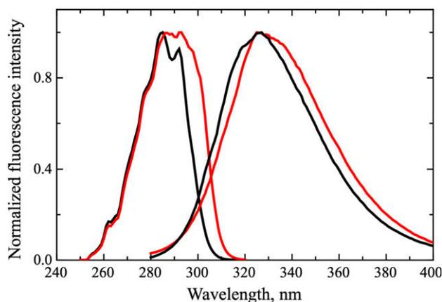
Fig. 2. Normalized steady-state fluorescence excitation and emission spectra of native WT apoflavodoxin (black) and native 5-FTrp apoflavodoxin (red). Apoflavodoxin concentration is 4  $\mu\text{M}$  in 100 mM potassium pyrophosphate, pH 6.0, 25 °C. The excitation wavelength is 280 nm for emission spectra. The emission wavelength is 330 nm for excitation spectra. The excitation and emission slit widths are 2 nm.
