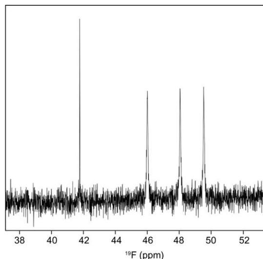
Fig. 1.  $^{19}\text{F}$  NMR spectrum of 5-FTrp flavodoxin in 100 mM potassium pyrophosphate, pH 6.0, at 25 °C. The resonance at about 42 ppm is due to the chemical shift reference 4-fluoro-phenylalanine.
