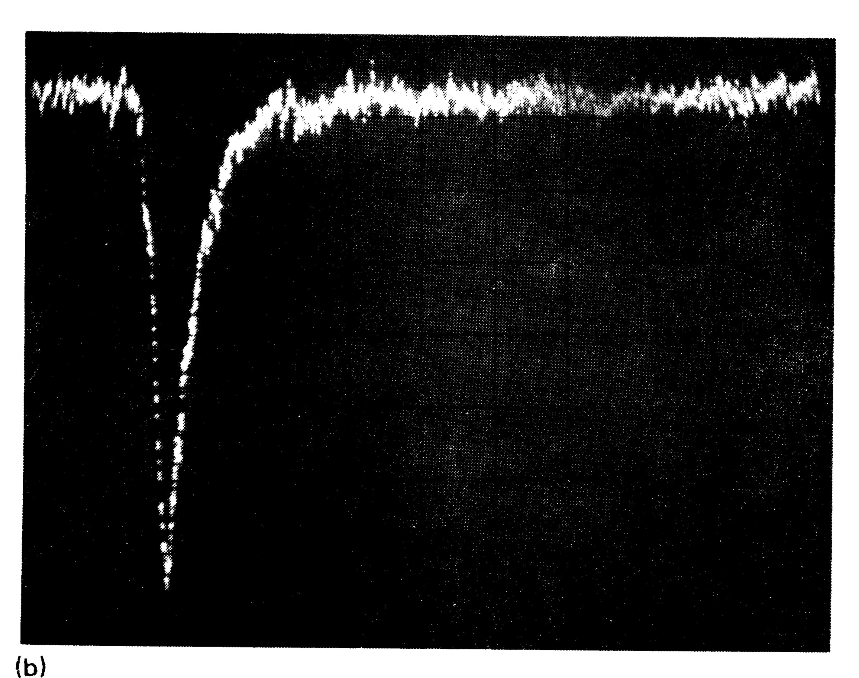
FIG. 4. Pulse shapes on the display of a sampling oscilloscope from the output (514.5 nm) of a mode-locked Ar-ion laser, detected with Telefunken BPW 28 photodiodes in a home-built mount. The optical substrates were rotated 45° around a vertical axis (a) and about 57° around a horizontal axis (b).
