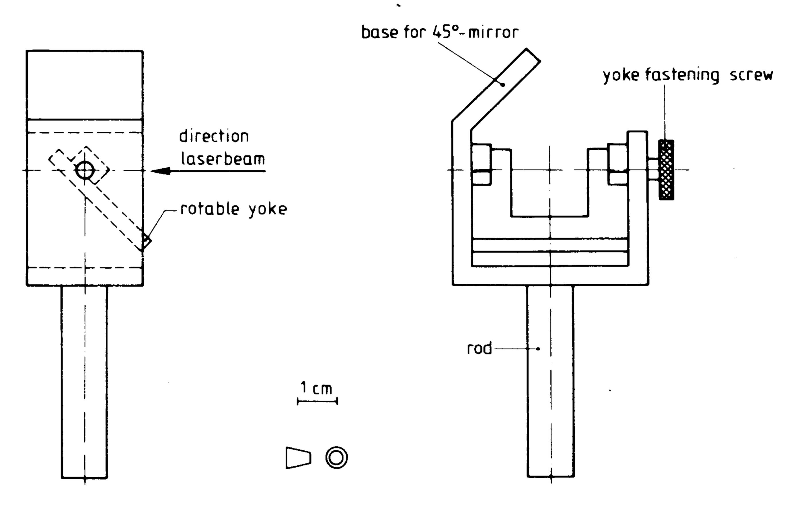
FIG. 3. Beam-splitter design.
