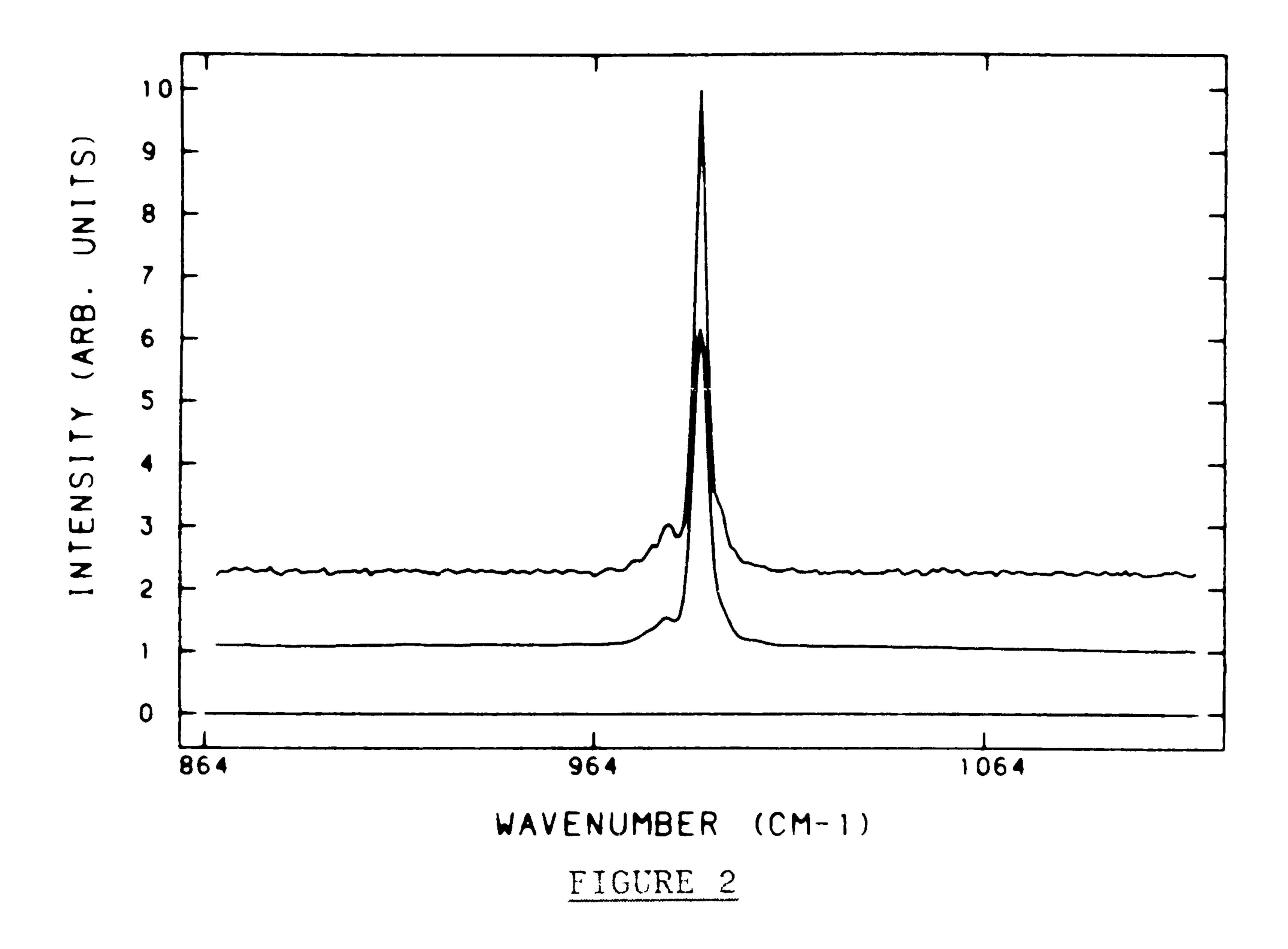
Raman spectrum of benzene either synchronously detected (SD, upper trace) or with photon counting (PC) detection (lower trace)
