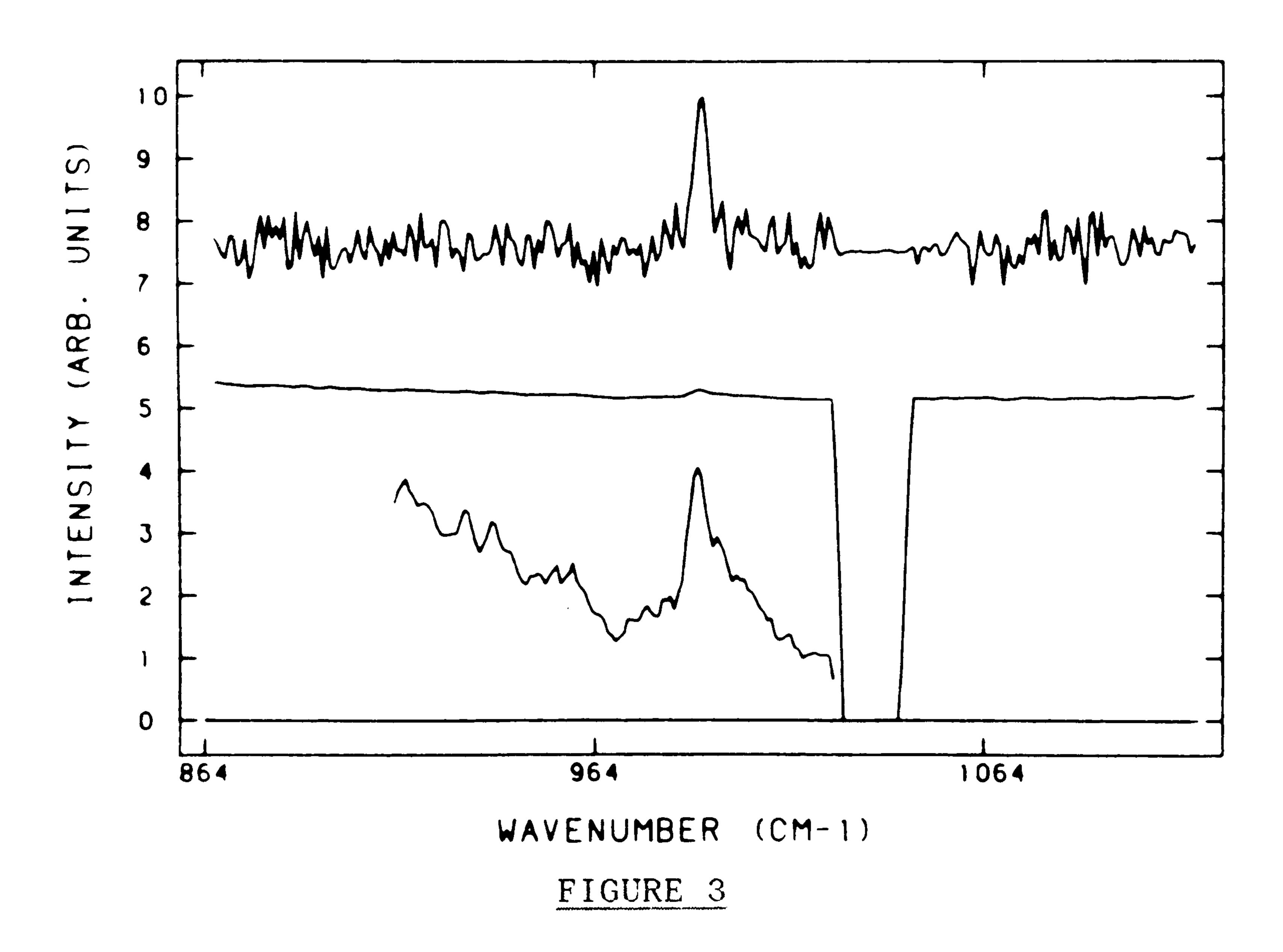
Raman spectrum of benzene doped with 20  $\mu$ M MLF, SD scan upper trace and PC scan lower trace. The inset is a scaled up fragment of the PC scan (see text). In the case of a shut-off of the laser light the PC spectrum goes to zero and the SD spectrum remains unaffected but the noise level is decreased.
