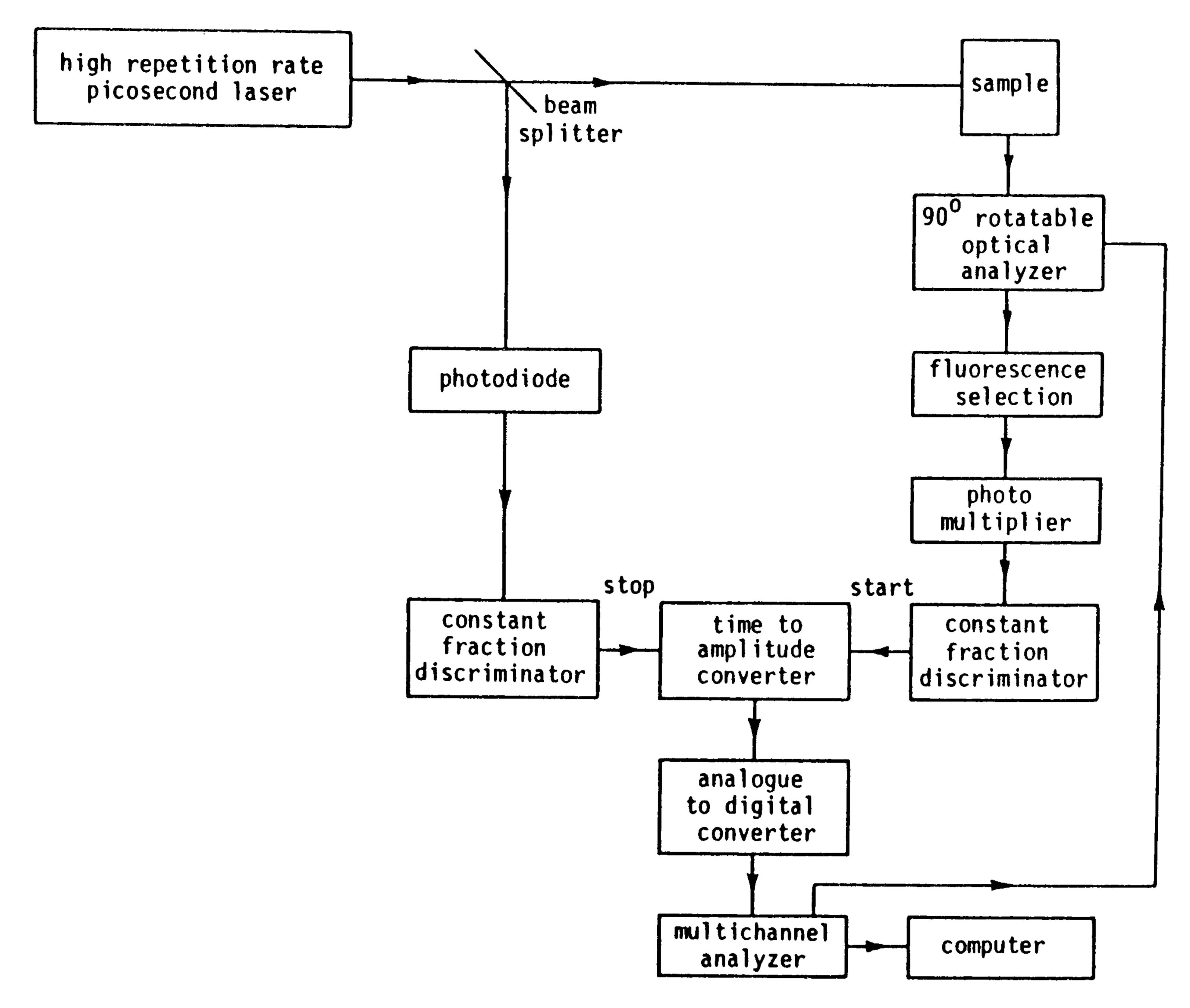
Fig. 1. Block diagram of the experimental setup.
