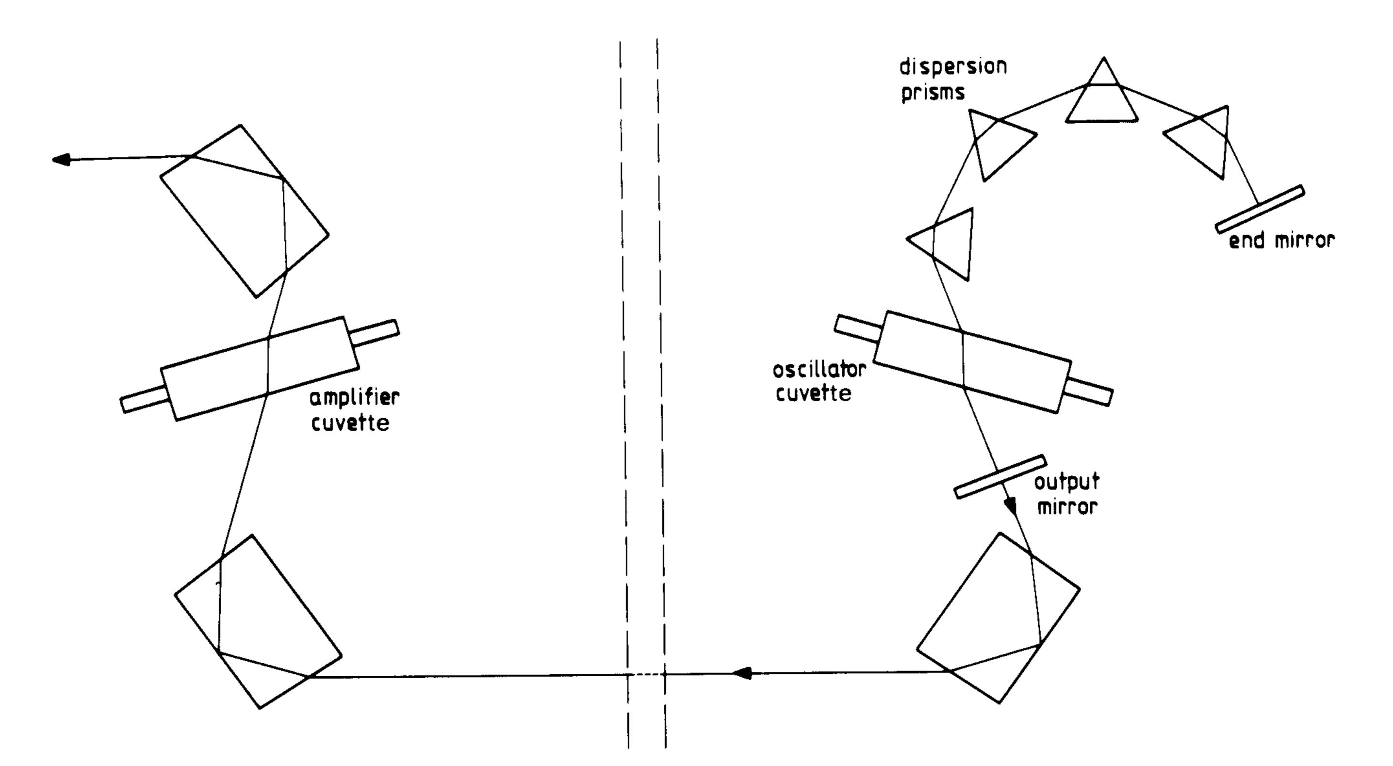
Fig. 3. Layout of the oscillator-amplifier scheme.
