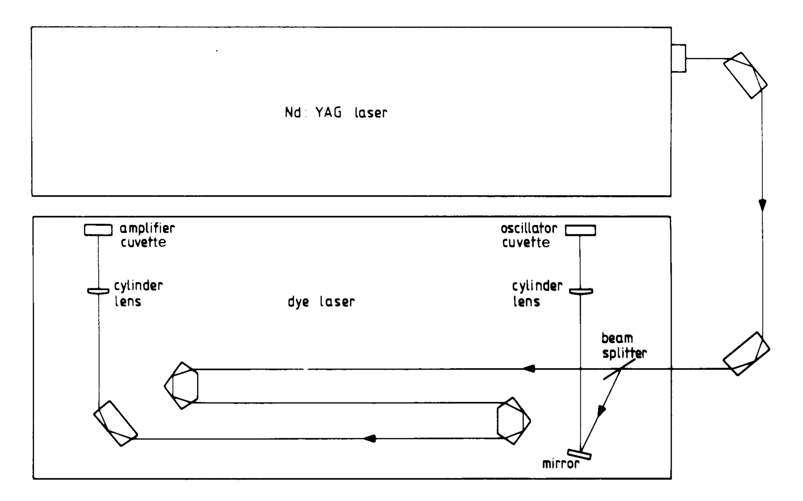
Fig. 1. Layout of the pump scheme.
