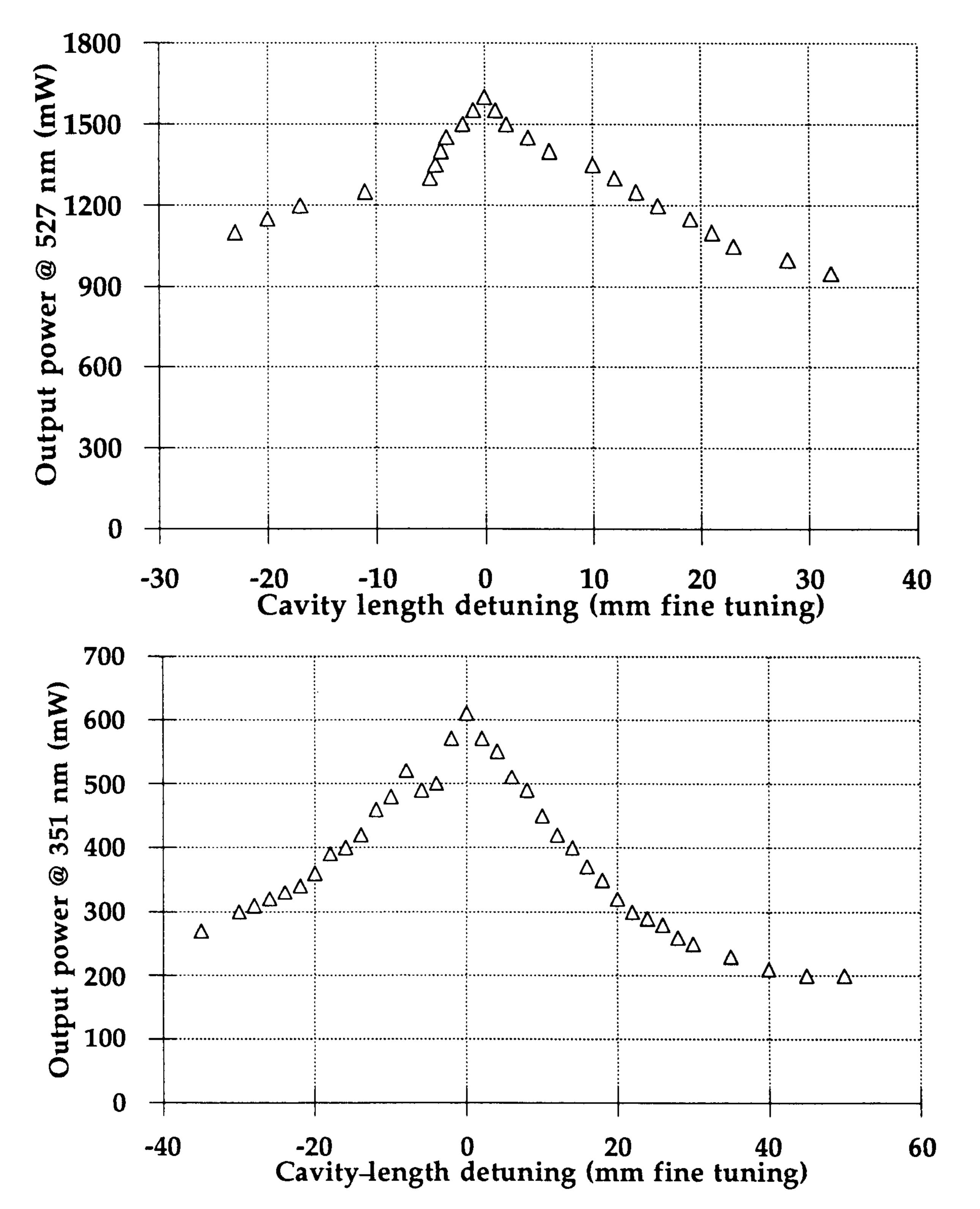
Fig. 1. Output power after frequency doubling and tripling following manual cavity-length detuning.
