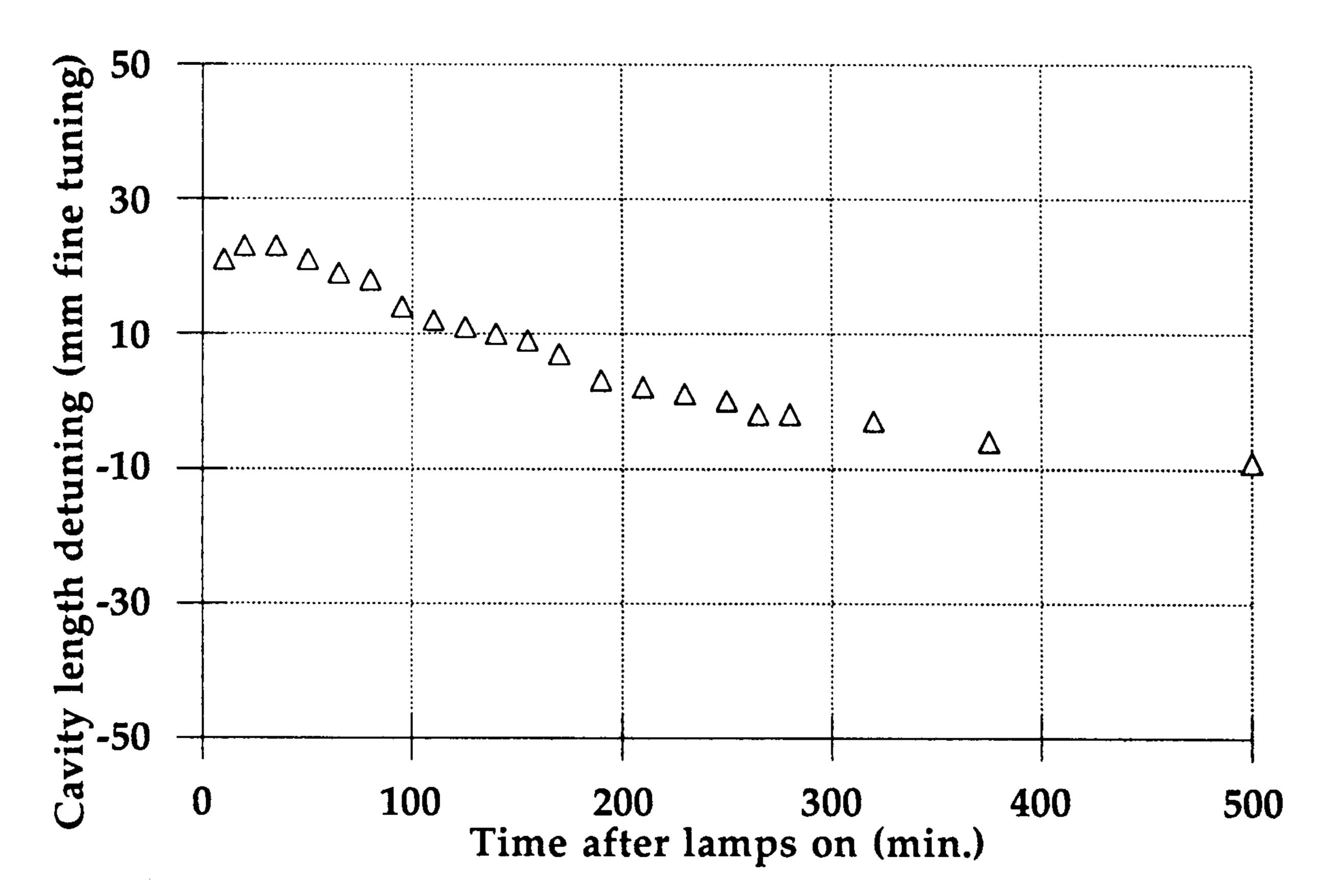
Fig. 2. Cavity-length detuning that is due to heating effects caused by dissipation after the lamps are switched on.
