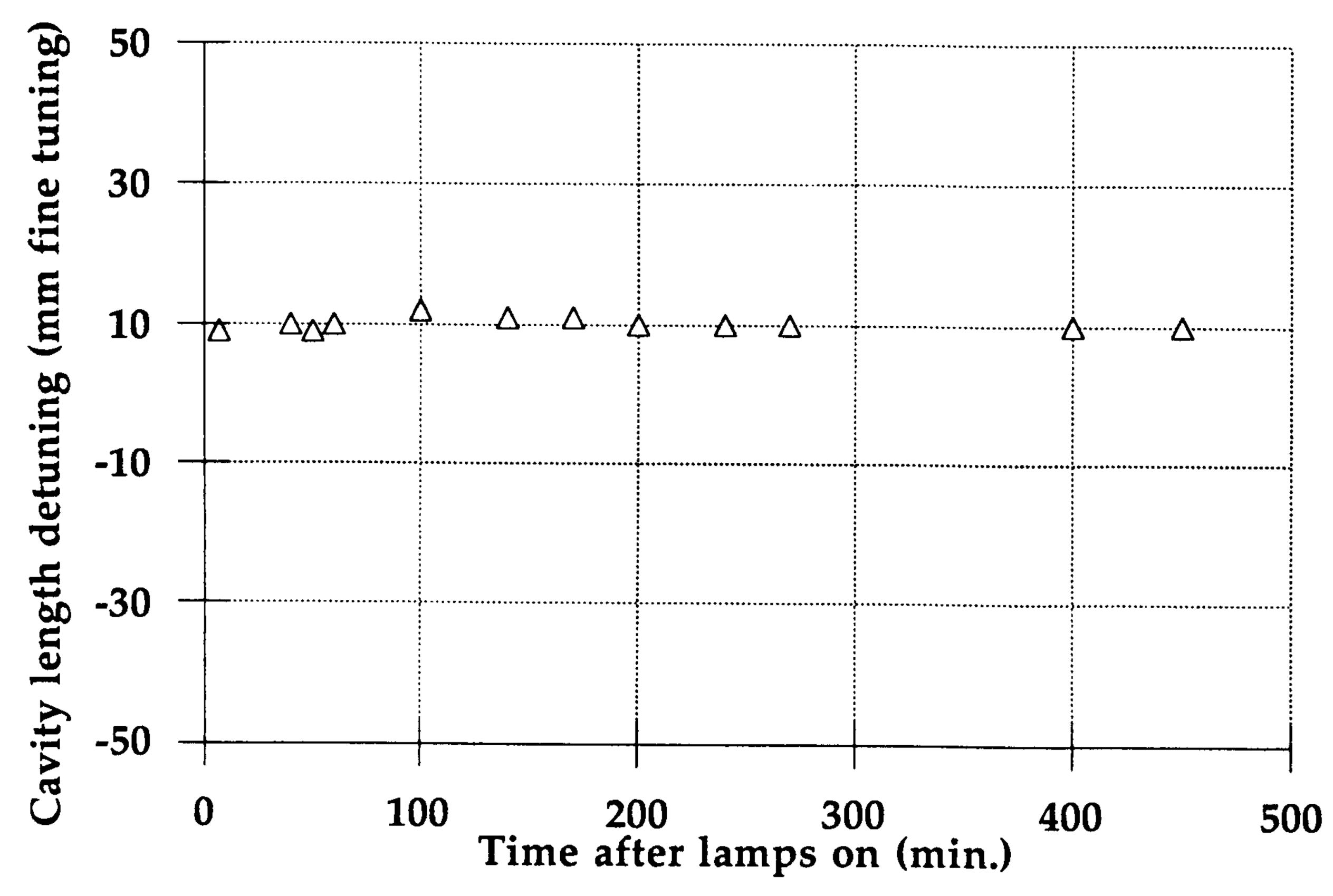
Fig. 3. Cavity-length detuning after the lamps are switched on and controlling the artificial heater, as described in the text.
